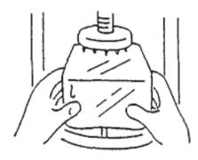
3. Turn the Ice Block Holder Crank counter-clockwise to lower the Ice Block Holder onto ice. Apply pressure until the Ice Block Holder prongs are firmly imbedded in the ice. The polycarbonate shield should be turned horizontally to the front.
