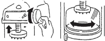
2. Make sure that the blade is in the down position, below the Shaving Plate opening. Place ice block flat side up, and center on the shaving plate. This may require a couple of tries.
