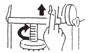
5. Turn the Blade Adjustment Knob located on the left side of Shaving Plate Frame counter-clockwise SLOWLY. This will raise the blade, allowing it to shave the ice. The higher the blade is raised, the coarser and faster the ice will come out.
